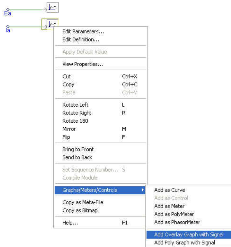
Fig.2 Basic steps to create a graph with a selected signal.
