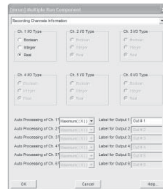
Data sheet for Multiple Run component defining the recording channels information.
